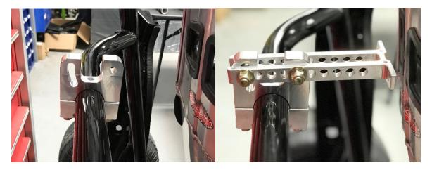
Rotating the crossbar clamp 180 degrees to the top will come in handy if your vehicle's crossbar is lower, or the height of your seat is higher. We realize not every seat mount arrangement is the same, and our Billet Upper Adjustable Seat Mount reflects that thought. It is truly designed and built to fit a wide variety of seating solutions.
