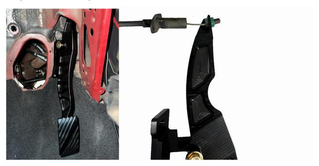
If you have an aftermarket adjustable cable, please refer to your throttle cable manufacturer's installation instructions. DO NOT floor your pedal without making sure your cable is set up properly, or you can break your throttle cable.
