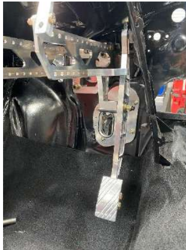
The completed throttle pedal assembly will look as shown here.
