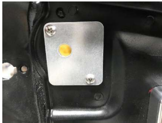
The throttle cable firewall bracket uses the factory clutch cable opening in the firewall. There is already one hole that is used to secure the factory clutch cable, so you must make another hole for the throttle cable firewall bracket. This picture was taken while facing the firewall.
