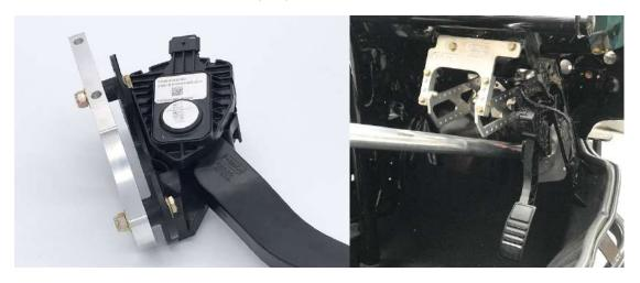
With a 1979-1993 Mustang, it may be necessary to modify or trim the factory cowl support bracket. However, that is only if you mount the pedal to the point where it is up against the firewall. The factory cowl support panel curves in towards the pedals, and the panel and pedal are fighting for the same space. This bracket is the one attaching the cowl to the trans tunnel under the dash
