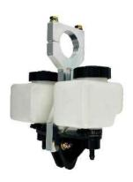
The main structure/brake pedal assembly includes this reservoir mount for the brake master cylinder. This mount is deigned to use the roll bar running behind the dash, but if you don't have that, the reservoirs still need to be mounted above the master cylinder for proper operation as they are gravity fed.
