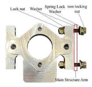
The clutch sub-assembly attaches to the main structure arm in the orientation pictured above. We recommend installing the set screw, washer, and locknut while the sub-assembly is outside the car. Make sure some of the set screw protrudes through the locknut to ensure the nylon lock is engaged. Once that is built, slide the set screws through the main structure arm and use the washer, spring lock washer, and non-locking nut to fasten it to the main structure.
