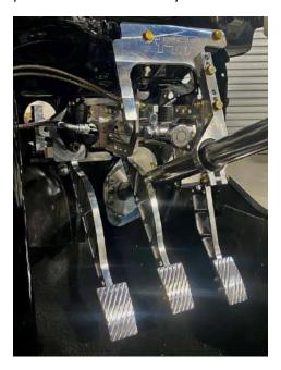
Use the hardware marked Pedal Pads to attach the pedal pad to the clutch pedal, and you are done. The completed clutch pedal assembly is probably the last subassembly installed onto the pedal assembly. As you can see, all lines are connected and routed to the bulkhead at the firewall.
