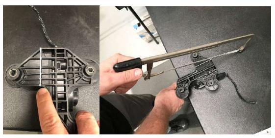
To add our Coyote Swap Pedal Bracket to the factory or Control Pack pedal, the factory bracket must be modified. We eliminate the 3<sup>rd</sup> hole on the factory pedal. We make a mark on the factory webbing where we need to cut it and use a saw to make the cut. The factory pedal is plastic, so this is a simple modification.
