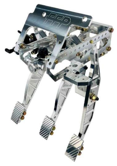
If you are reading this, you have already installed the FFP Customs pedal assembly's main structure, brake pedal subassembly, and most likely, the throttle pedal subassembly. The last piece of the FFP Customs patented pedal assembly is the clutch pedal subassembly. As we have mentioned, everything is built off the pedal assembly's main structure. As such, the clutch pedal uses the main structure as its attaching point.
