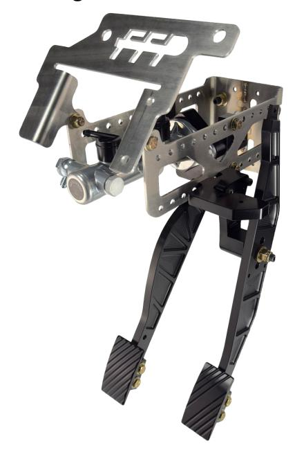
If you are reading this, you have already installed the FFP Customs pedal assembly's main structure and brake pedal subassembly. With that, you can move on to the throttle pedal subassembly. As we have mentioned, everything is built off the pedal assembly's main structure. As such, the throttle pedal uses the main structure as its attaching point.
