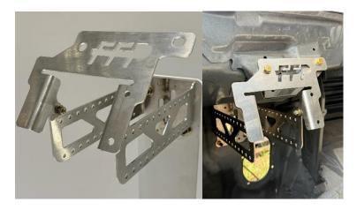
The Pedal Assembly's main structure installs using the outside firewall mount and the inside firewall mount. The main structure is the building block of the pedal assembly. Everything is built off the main structure. The main structure bolts to the firewall and the cowling area under the dash. The cowl mount is part of the main structure and that part bolts the main structure and cowling area. Then the brake master cylinder and brake pedal are attached to the main structure in the center.
