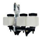
The Reservoir Mount either attaches to the roll bar, or you can remotely mount the reservoirs, but they must be mounted above the master cylinder since they are gravity fed. The Wilwood instructions go over this, as well as the bleeding procedure. The picture to the right shows an example of how you can add the clutch reservoir tank to the existing brake reservoir tanks.
