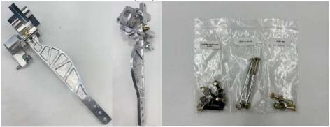
The clutch pedal is sectioned off by itself in the box when you receive the pedal assembly. It uses a mount like that of the brake pedal to attach it to the main structure. We include labeled hardware bags for the pedal pad, reservoir mount, and clutch master cylinder mount.
