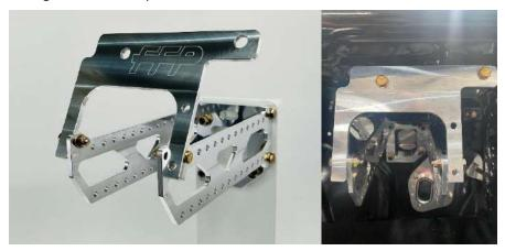
The Pedal Assembly's main structure installs using the outside firewall mount and the inside firewall mount. The main structure is the building block of the pedal assembly. Everything is built off the main structure. The main structure bolts to the firewall and the cowling area under the dash. The cowl mount is part of the main structure and that part bolts to the main structure and cowling area. Then the brake master cylinder and brake pedal are attached to the main structure in the center.
