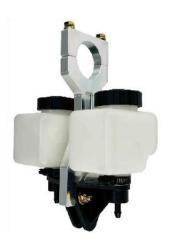
The main structure/brake pedal assembly includes this reservoir mount for the brake master cylinder. This mount is designed to use the roll bar running behind the dash, but if you don't have that, the reservoirs still need to be mounted above the master cylinder for proper operation as they are gravity fed.
