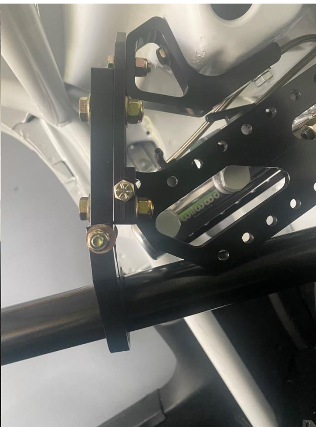
Since the cowl Panel mount is thicker where the bottom bolt of the upper steering column mounts, the longer bolt must be used in the lower mounting hole
