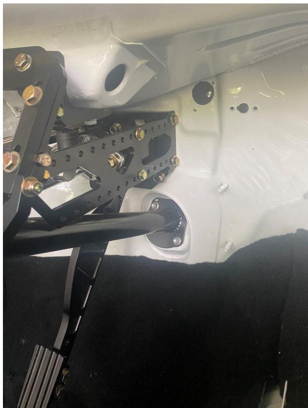
The steering column is mounted in the proper orientation when the round edge of the firewall mount flange is facing the bottom left corner. Shown at highest setting
