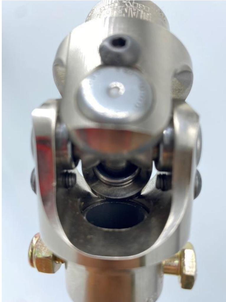
Here you can see how the chromoly steering shaft is inserted and through bolted to allow full articulation while still engaging as much of the shaft as possible
