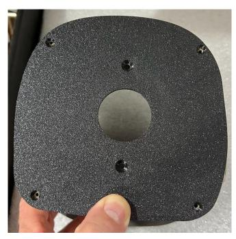
Once you have your 4 mounting screw holes drilled, you can now move on to mount your factory multi-function switch to our steering column clamp using the included 10-32 bolts and 10-32 locknuts. The orientation of the switch after it is installed can be seen in the picture below.
