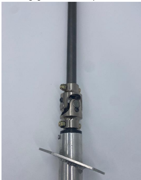
Notice the small gap between the steering bushing and the joint, this prevents full disengagement of the shaft if your set screw were to fail (STEERING JOINTS NOT INCLUDED)
