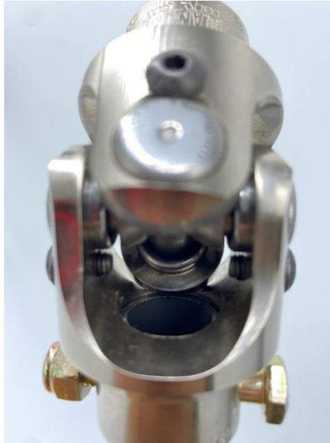
Here you can see how the chromoly steering shaft is inserted and through bolted to allow full articulation while still engaging as much of the shaft as possible (STEERING JOINTS NOT INCLUDED)
