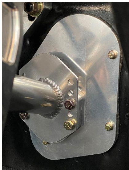
Firewall Mount installed on our display cart at its highest setting (inside view)
