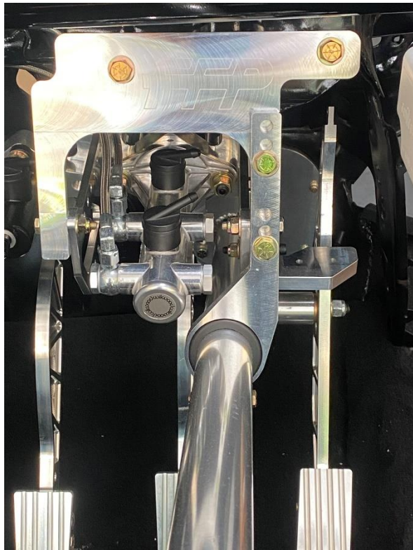
Our Upper Steering Mount properly mounted to our adjustable pedal assembly at its highest setting
