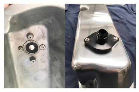
The valve cover we're using in these photos already featured a grommet hole, and as you can see, it's more than enough for both the -10 and -12 AN Fittings. The rubber part of the washer needs to be against the bottom side of the valve cover, while the rubber O-ring needs to be inserted into the bottom of the fitting before it is mounted to the valve cover.
