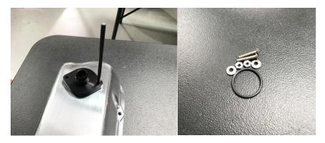
Once you have decided where to mount the fitting, use a punch to mark the hole location for the hardware. Then use a Sharpie to trace the hole for the opening. The -10 AN Fitting hole is roughly half an inch, while the -12 Fitting hole is roughly 5/8-inch. Hardware for the AN Fittings is included, which entails buttonhead Allen bolts, rubber bonded washers, two nuts, and an O-ring.
