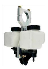
The main structure/brake pedal assembly includes this reservoir mount for the brake master cylinder. This mount is designed to use the roll bar running behind the dash, but if you don't have that, the reservoirs still need to be mounted above the master cylinder for proper operation as they are gravity fed.
