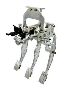
Use the hardware marked Pedal Pads to attach the pedal pad to the clutch pedal, and you are done. The completed clutch pedal assembly is probably the last subassembly installed onto the pedal assembly. All lines should be connected and routed to the bulkhead at the firewall.
