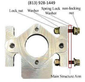
The clutch master cylinder mount uses 2 set screws, 2 lock nuts, 2 spring lock washers, and 2 nuts in the orientation above to mount to the main structure.
